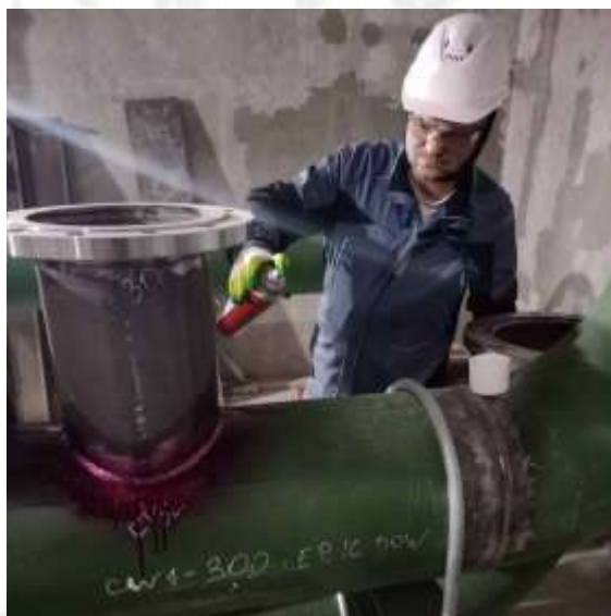
3-rasm. Kapillyar nazorat usulida penetrant suyuqlik yordamida tekshiruv
