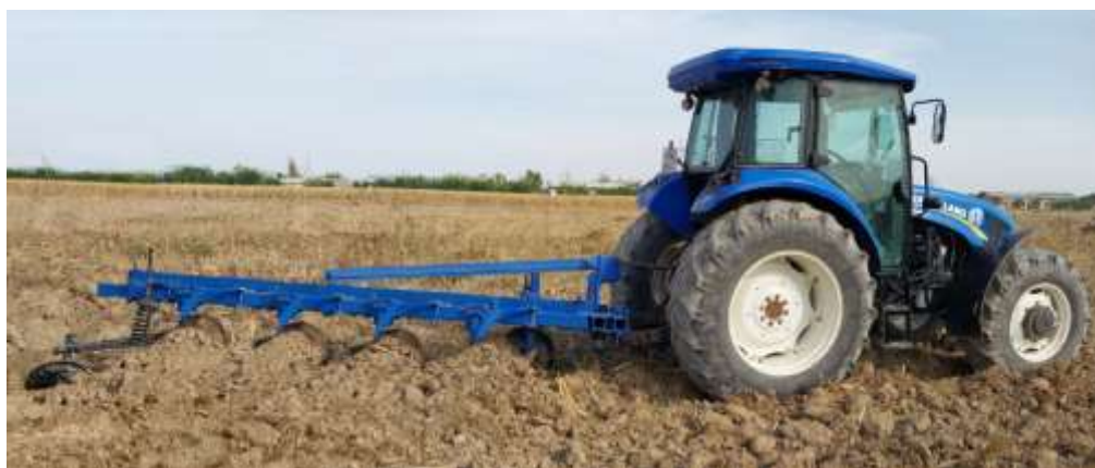
Figure 1. View of the Operating Process of the Disc Plough Equipped with a Scraper
