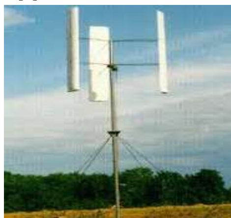
4-rasm. a) Sistan tipidagi vertikal o'qli shamol generatori b) H-rotor dizaynidagi shamol turbinasi
