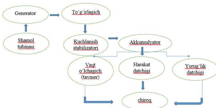
5-rasm. Verikal o'qli shamol turbinasining energiya chiqarish printsiplining ishlash sxemasi
