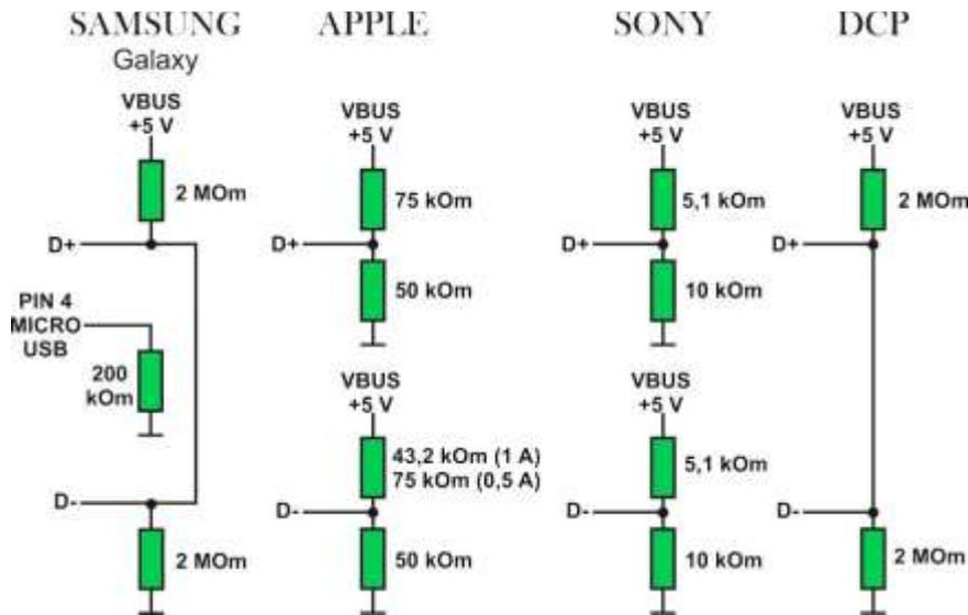
**Figure 2. Setting resistor dividers to establish specific voltage levels on the signal lines of charging devices from leading manufacturers**
