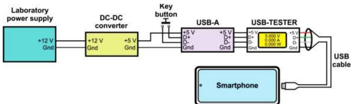
**Figure 1. Experimental circuit for observing the operation of a QC 2.0 standard charging device**
