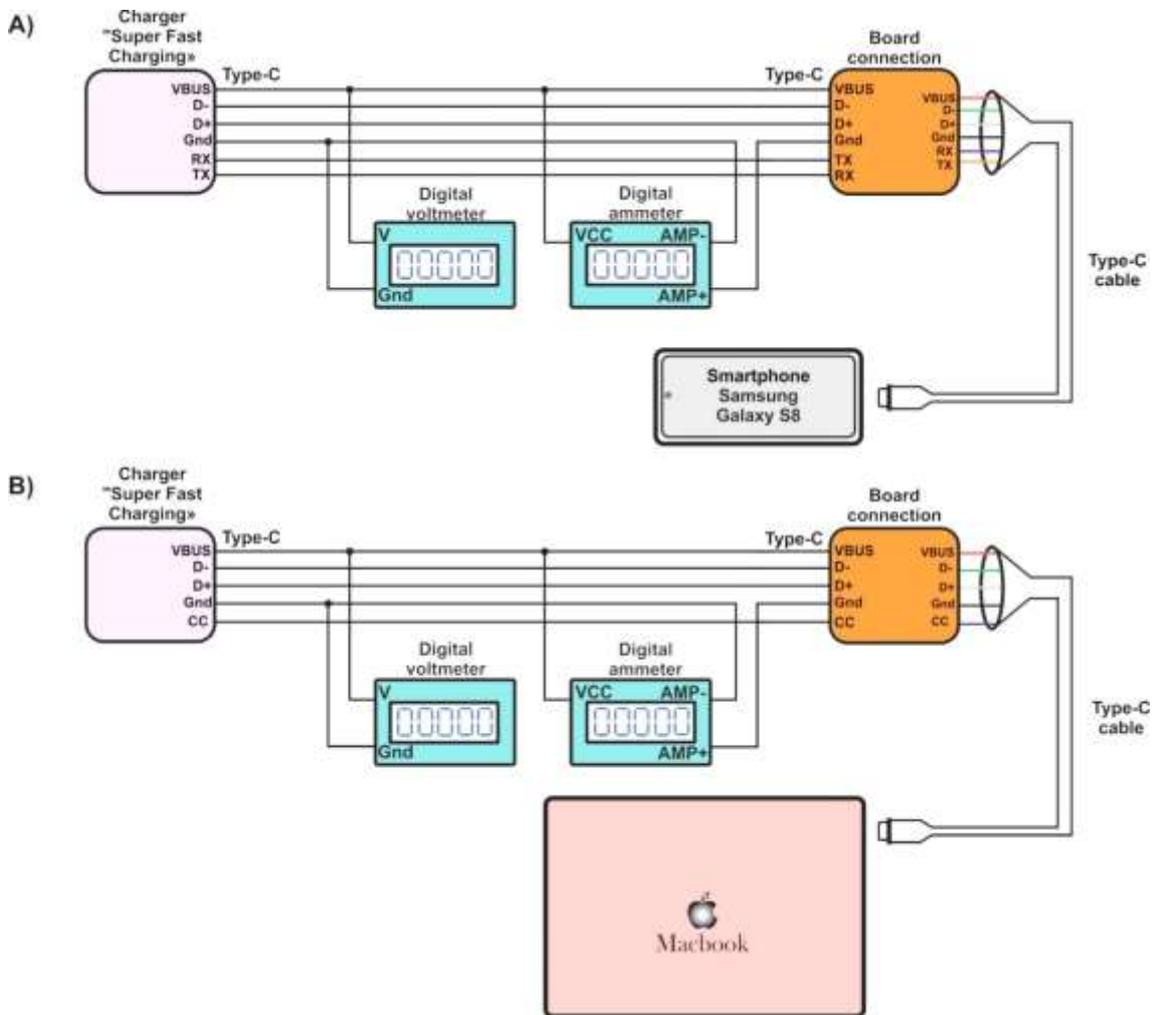
**Figure 3. Investigation of smart devices using the Power Delivery connection standard**
